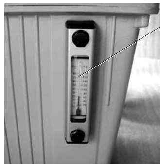
Fig. 21: Oil temperature and oil level
